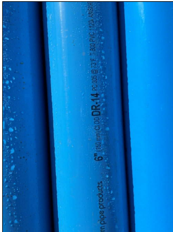
Figure 2: 6" C900 to be installed
